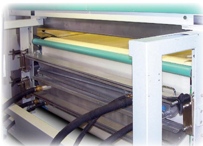
Details of lacquer recovery device for belt-cleaning "wet on wet" (patented).
