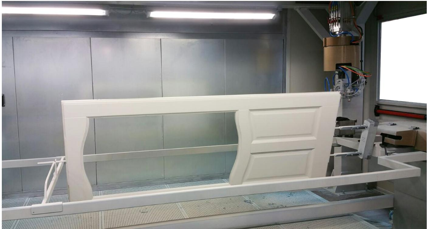
Door and window rotation system with the possibility to remove the support for drying on trolleys.
